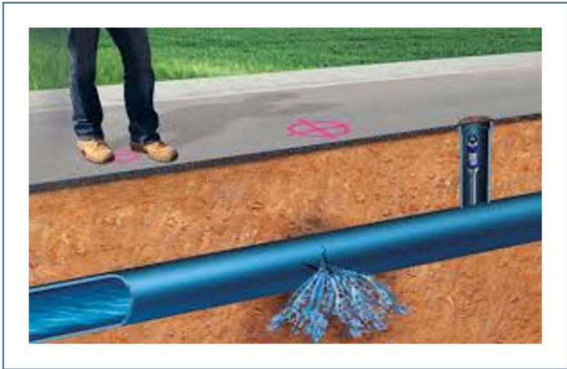
Figure 4.5: Invisible water leakage at the detected fault location [Internet]
