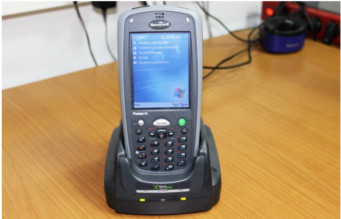
FIGURE 3.3: A MOBILE DEVICE FOR COLLECTING METER READINGS (DOLPHIN 7900)
