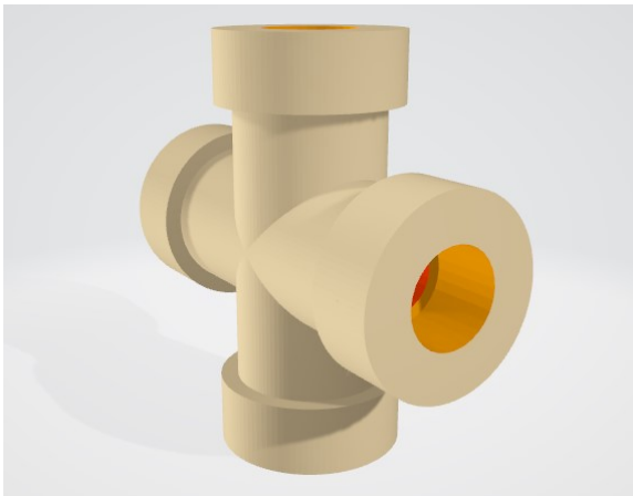
Figure 19 Equal Cross Body generated from CSG code
