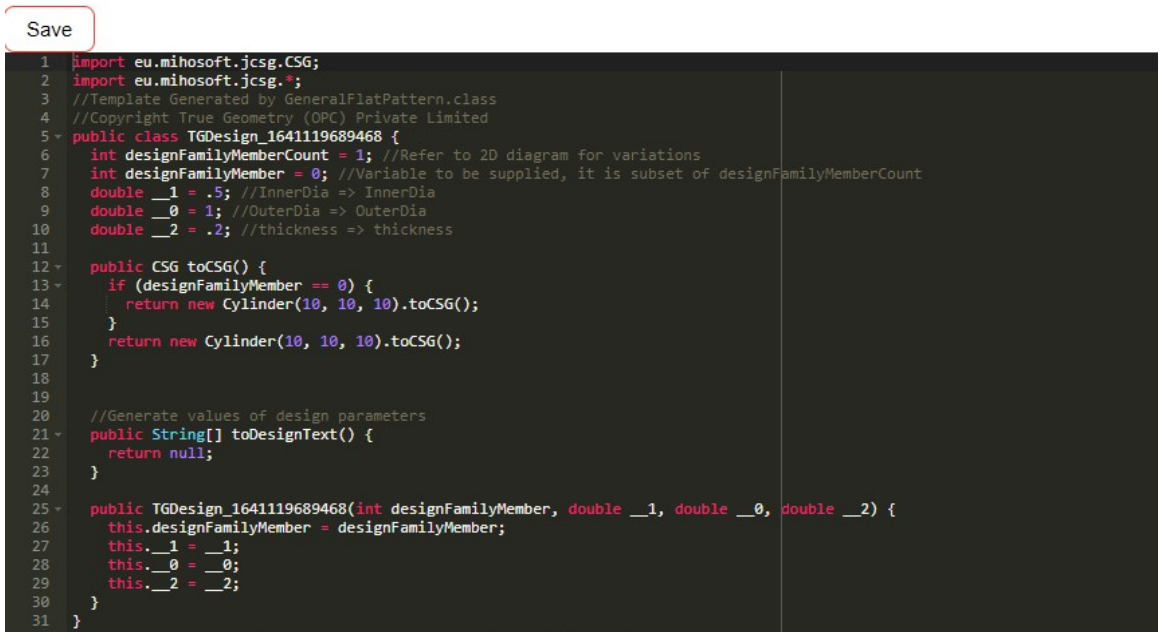
Figure 14 Code template generated from ICARE formal model Then the code is modified as shown below:
