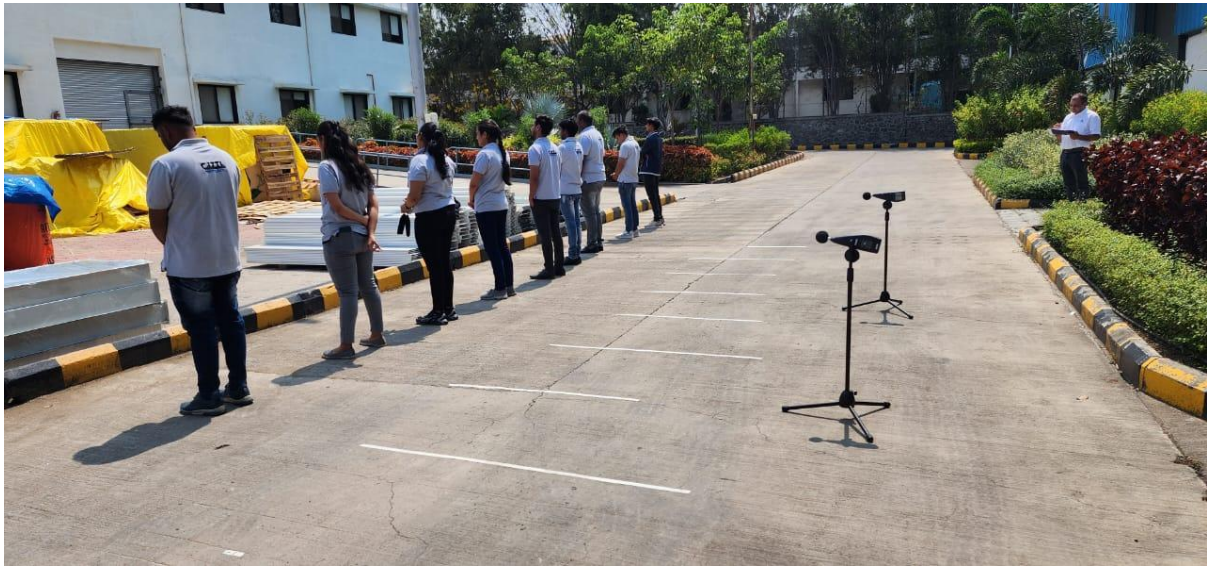
Figure 41: Experimental scene of Intensity of Sound (IS) Versus Audibility Distance (AD) wherein participants are standing in a row at a gap of 1 meter from each one.
