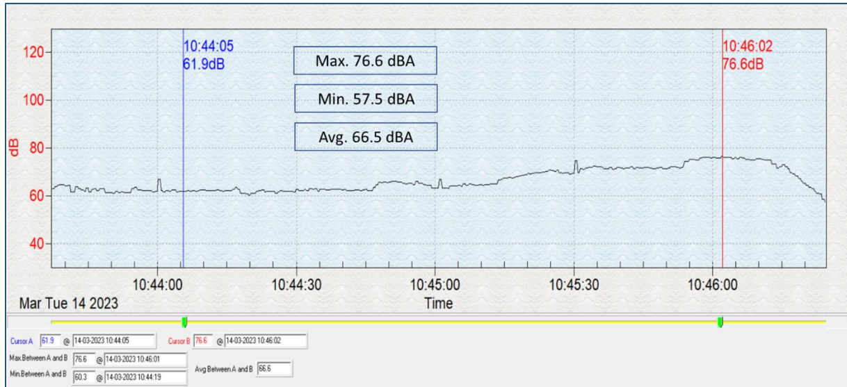
Figure 67: Sound dBA graph for test-1 for Honda Activa ICE Scooter by sound meter-2 at 3m distance
