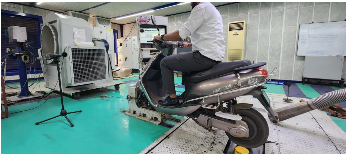
Figure 39: Sound level testing in Lab of EV Hero Electric Scooter at variable speeds with the help of sound meter placed at a distance of one meter from the vehicles.
