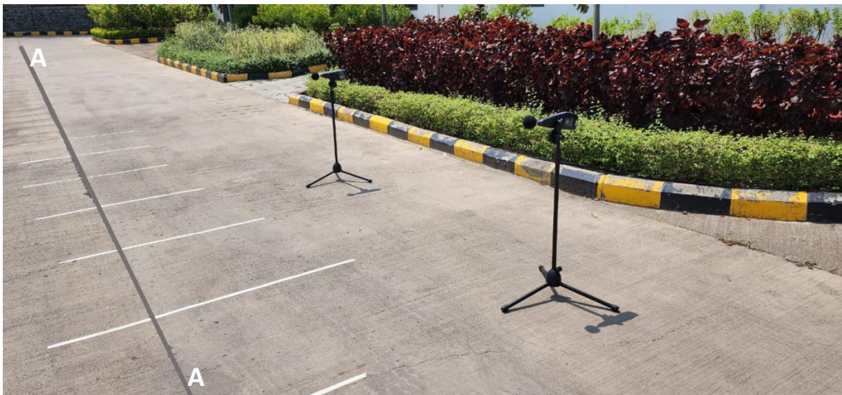
Figure 40: Experiment setup for Intensity of sound (IS) Versus Audibility Distance (AD) with masking tapes at one meter distance to calculate the vehicle distance.
