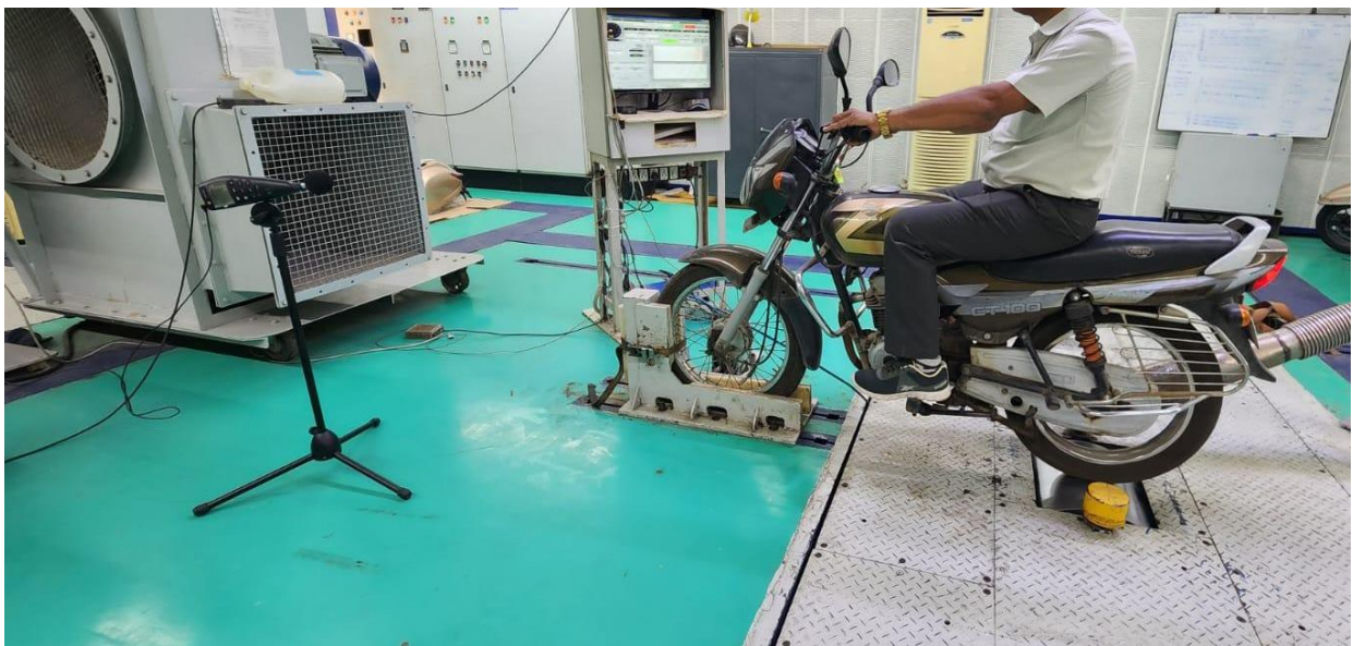
Figure 37: Sound level testing in Lab of ICE Motorcycle at variable speeds with the help of sound meter placed at a distance of one meter from the vehicles.
