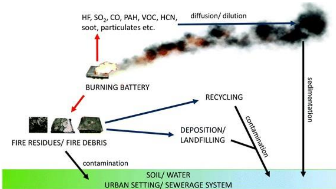
FIGURE 5. EMISSION PATHWAYS FROM FIRES (STEC ET AL., 2019)
