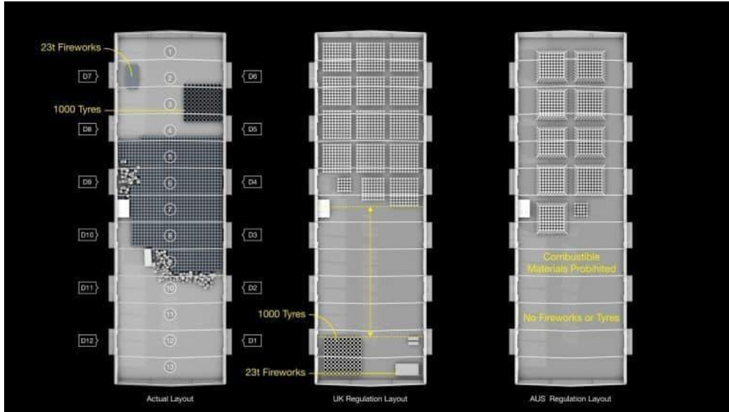
Figure 12: Incorrect Hanger 12 Layout of Ammonium Nitrate in Beirut v British and Australian Dangerous Goods Standards.
