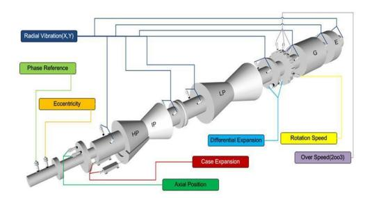
Figure 25 Turbo Supervisory Instrumentation-TSI
