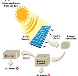
Source: Electricity generation: Shaikh, Mohd Rizwan et al (2017) Figure 13: Power generation from Solar energy.
