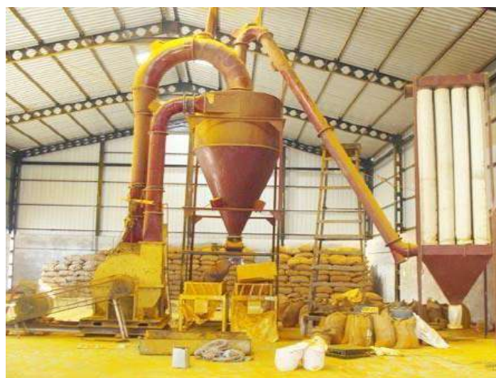
Figure No.3.35 Turmeric grinding unit
